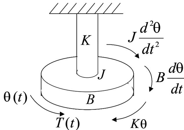
$T_m(t)$  = motor torque;  $J_m$  = motor inertia;  $B_m$  = motor viscous friction coefficient;  $J_L$  = load inertia,  $K$  = spring constant of the shaft;  $\theta_m(t)$  = load displacement;
